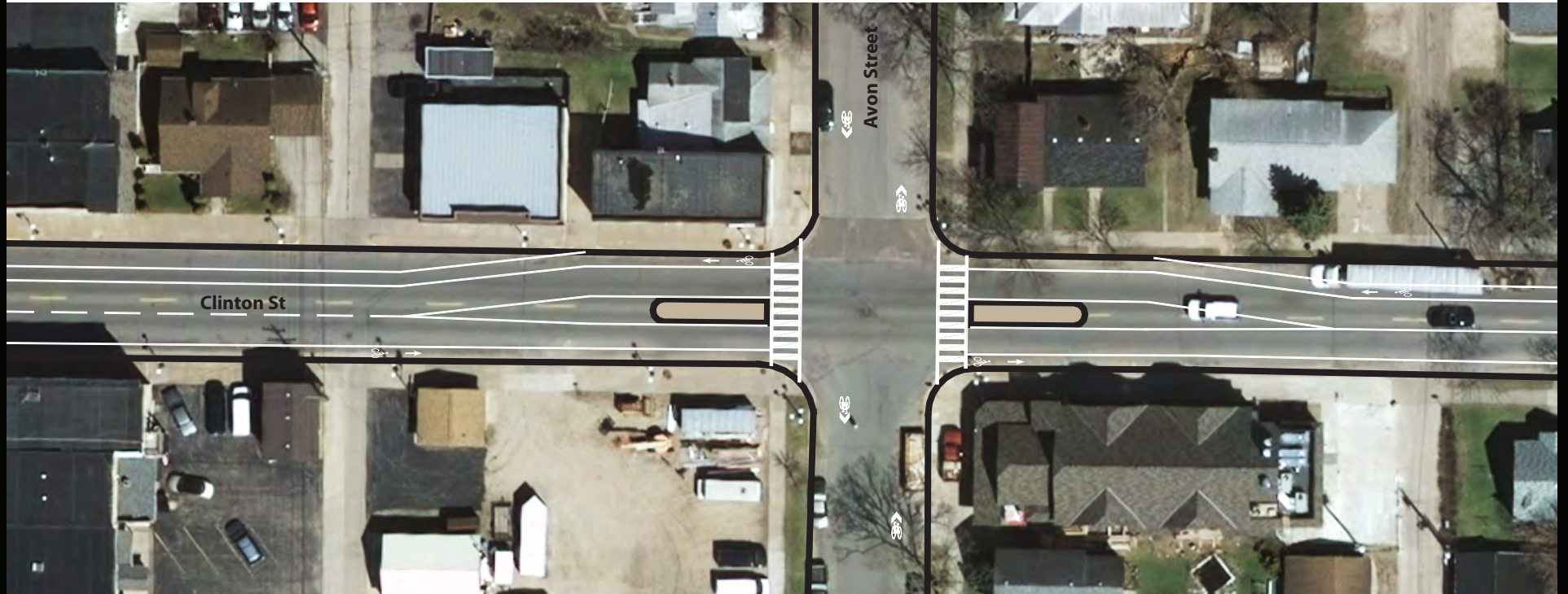
Short Term Option: Add Pedestrian Refuge Islands to Improve Bicycle Crossings Along the Proposed Avon Street Bicycle Boulevard
