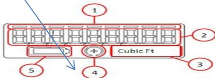
**\*\*\*WHEN READING 1 1/2" TO 10" SENSUS OMNI C<sup>2</sup> METERS, THERE ARE 3 DIFFERENT SCREENS DISPLAYED. EACH TIME THE REGISTER LID IS OPENED OR CLOSED; YOU WILL SEE THE WORDS, AMR, TOTAL OR TEST ABOVE THE NUMBERS.**
